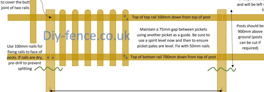
Posts should be concreted 3.0m apart from centre points of the posts. Posts should be in the ground roughly 600mm. A minimum of 450mm should be achieved for picket fencing. Posts can be cut to suit.
