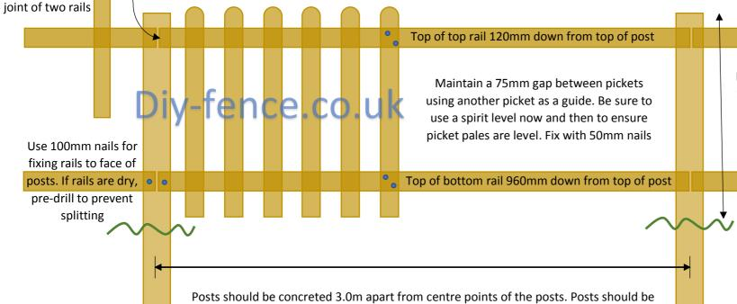
in the ground roughly 600mm. A minimum of 450mm should be achieved for picket fencing. Posts can be cut to suit.
