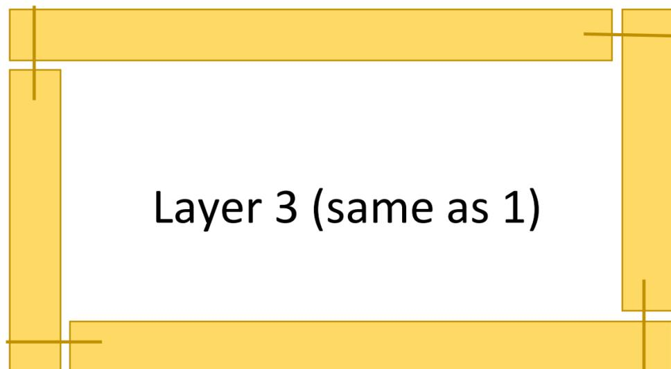
— Use hex head provided to screw structural screws through the pre-drilled holes. There is only one hole on each section of wood. Make sure all prominent holes are on the outside, not inside of the bed. Depending on the size kit ordered, you will only have two different lengths of timber if not one. Each piece can fit anywhere.
