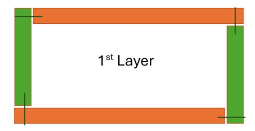
Use hex head provided to screw structural screws through the predrilled holes. There is only one hole on each section of wood. Make sure all prominent holes are on the outside, not inside of the bed. The colours indicate matching size timbers. Some layers may use 4 pieces the same size depending on size kit ordered. Check which size kit you ordered.
