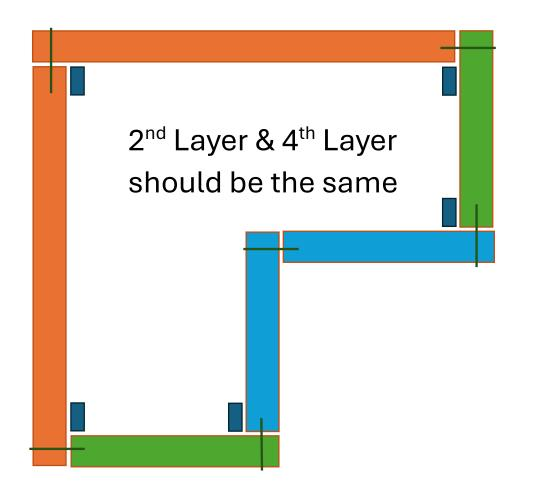
Layer 1 and 3 should be made the same, layer 2 and 4 should be made the same. The difference between them is that you start laying them the opposite way as before so that the joins are never in the same place.
